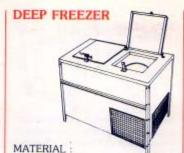
Inner tank is made out of 14 gauge Aluminium sheet outer of 16 gauge stainless steel, having 4" thick thermocole insulation sealed with bitumen.
