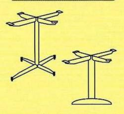
A commonly used stand made out of M.S. structural steel or stainless steel with vertical sturdy pipe support. The stand has got leveling screws. The top of different materials can be fixed as per choice. Available in different sizes with painted or powder coated finish.
