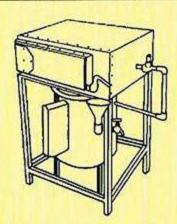
Boiler is out of 6 mm plate where steam is generated. The steaming pot is made out of stainless steel with tray arrangement with a lockable door. The steam from the boiler is admitted in the chamber through pipe with insulated cover. Available in two sizes for 60 or 120 Idlies at a time.
