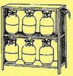
The cylinders are required to be stocked in open area hence for security and handling purpose this cage is required. The basic features are structural steel frame with lockable doors with a sheet top and sides covered by weldmesh. Available with 4/6/8/12 cylinders capacity.
