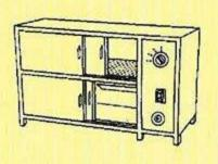
Generally this unit is tailor made according to the size required by the client to suit space and need. The unit is having 18 gauge S. S. sliding doors with 2 under shelves. Heaters with thermostat control indicator light and total side insulation to prevent heat loss are unique features.
